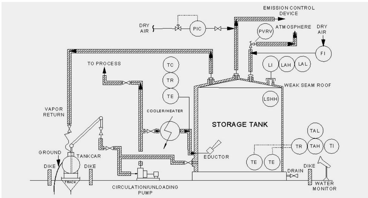
**Figure 12-2: Example of a Methacrylic Acid Storage Tank Temperature Control System**
